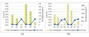
Figure 7: (a) Performance estimation errors of the pipeline structure model when mapping 6 DNNs onto Xilinx ZC706. N1~N3 represent AlexNet, ZF, and YOLO with 16-bit quantization, while N4~N6 represent the same group of networks using 8-bit quantization. (b) We swap the FPGA to Xilinx KU115 and evaluate the estimation errors on 8 DNNs where N1~N4 represent AlexNet, ZF, VGG16, and YOLO with 16-bit quantization while the rest 4 using 8-bit quantization.
