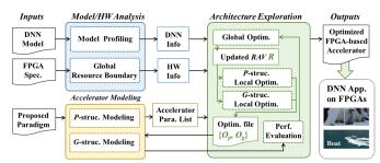
Figure 4: The Design flow of DNNExplorer containing 3 steps to generate optimized DNN accelerators given DNN models and FPGA specifications.
