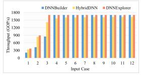
Figure 10: Throughput comparison when running VGG16 (batch size = 1) with 12 different input sizes.
