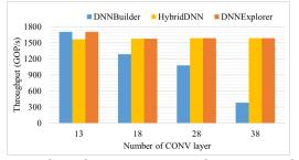
Figure 11: Throughput comparison when running deeper DNNs with the same  $3 \times 224 \times 224$  input.
