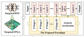
Figure 3: The proposed accelerator paradigm to overcome existing drawbacks when mapping DNNs onto FPGAs. It includes SP pipelined stages for layer  $1 \sim SP$  and a generic accelerator for the rest of layers. SP is the split-point.
