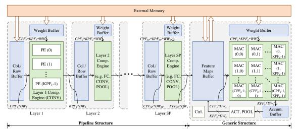
Figure 6: The proposed accelerator architecture with *SP* pipeline stages instantiated for processing the first *SP* DNN layers and a generic computation unit implemented for accelerating the rest of layers.
